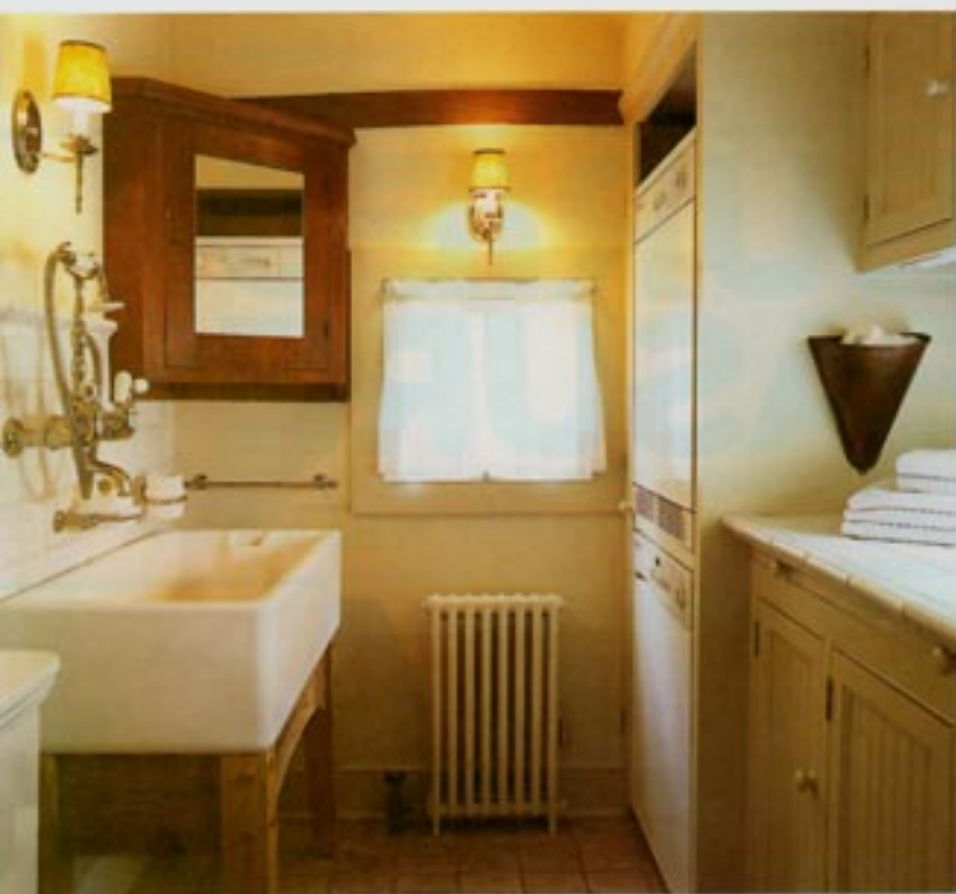
ABOVE: The half-bath-cum-laundry room on the first floor is completely new, but great care was taken to make the multifunctional space blend with the rest of the house. The old-fashioned farm sink is supported by a rustic, pegged mortise-and-tenon-legged stand that the homeowner built himself. BELOW: the house's exterior.
